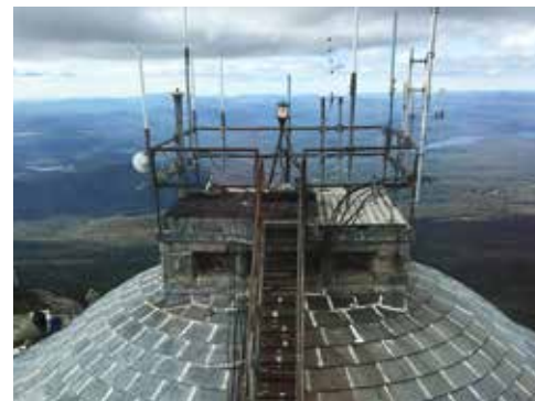
Cloud collection system and air quality monitoring on the summit of Whiteface Mountain
