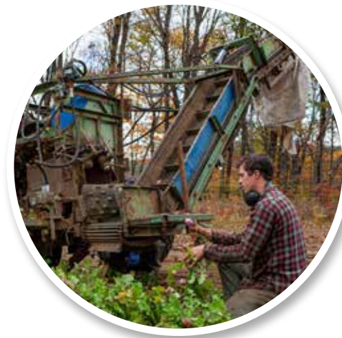
A conveyor harvester/cleaner for potatoes
