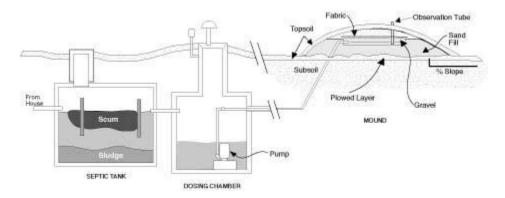
Mound Systems typically cost two to three times as much as a conventional septic system and require extra monitoring and maintenance. Source: Ohio State University Extension.
