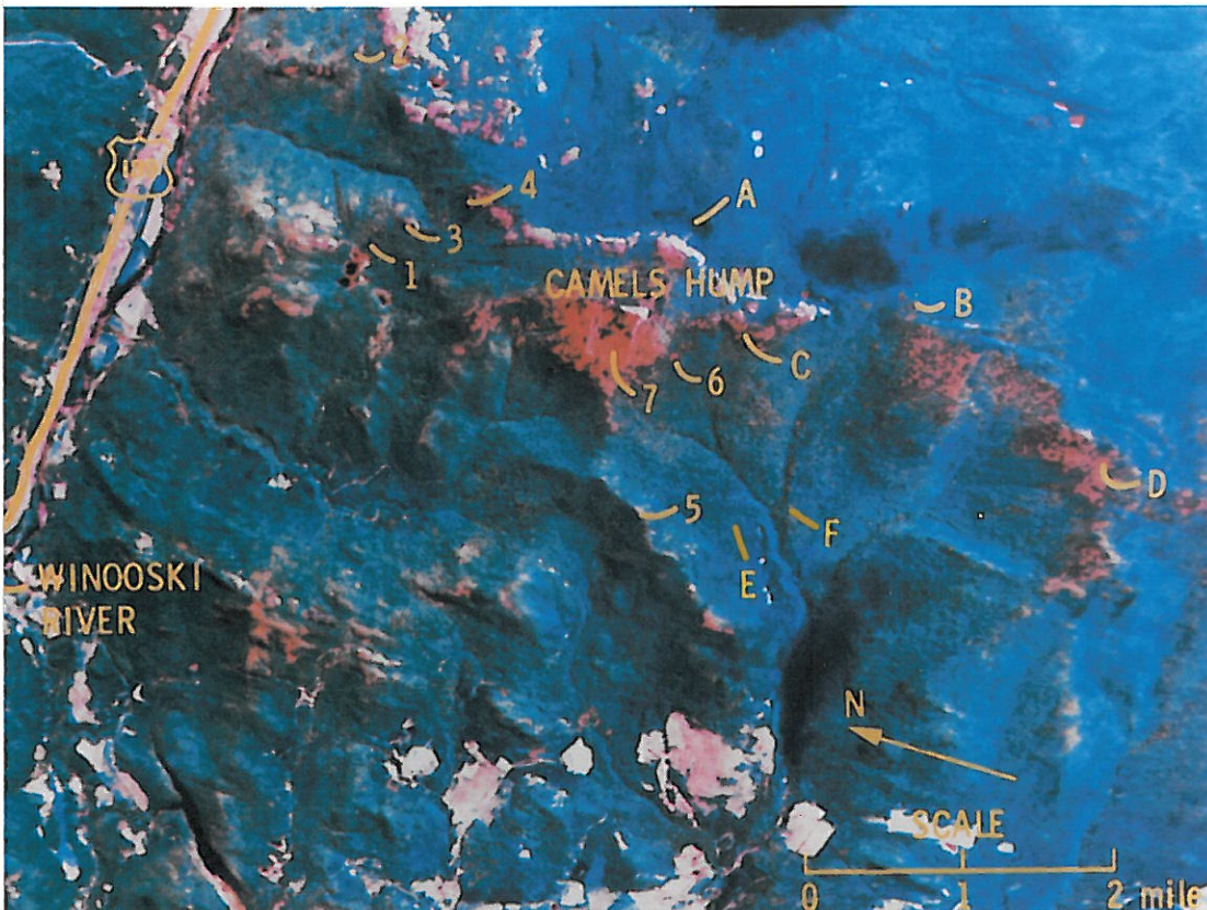
C Damage assessment impact of Camels Hump, Vermont, acquired 9/9/84. In this satellite image, healthy trees are depicted in light blue (hardwood species such as maple, beech, and birch) and dark blue (conifers such as pine and spruce/fir), while trees in decline are portrayed in orange, pink, and red (increasing levels of damage). Note that the highest damage at the upper elevations occurs on the west-facing slopes of Camels Hump and the mountains to the south. The numbered sites are the location of low damage (sites 1, 2, and 3), medium damage (sites 4 and 5), and high damage (sites 6 and 7) study areas selected on the basis of detailed ground assessment prior to the overflight. The lettered sites were selected for subsequent ground study. Sites A–D are conifer areas while E and F are hardwood stands.
